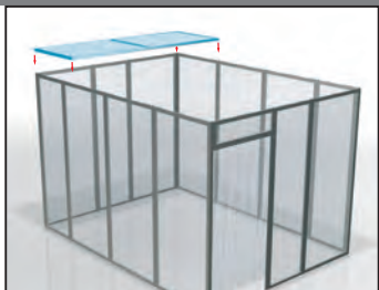
7 CEILING ELEMENTS ARE ASSEMBLED
