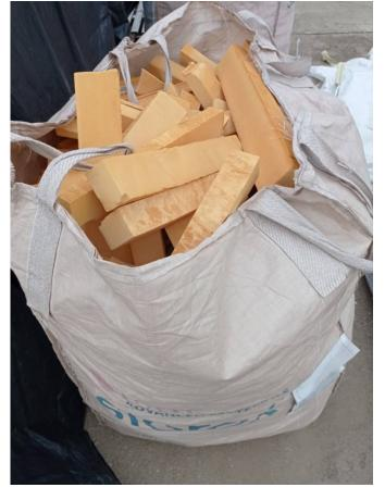
Currently, there is only one common method for the mechanical upcycling of rigid polyurethane foams. This process consists of grinding the waste foam into a fine powder and using it as a filler (max. 20%) in polyurethane products. At present, the rigid PU foams recovered from disposed household refrigerators and freezers are recycled in this way. However, it is important to note that most rigid PU and PIR foam waste is typically treated by incineration for energy use or deposited.
